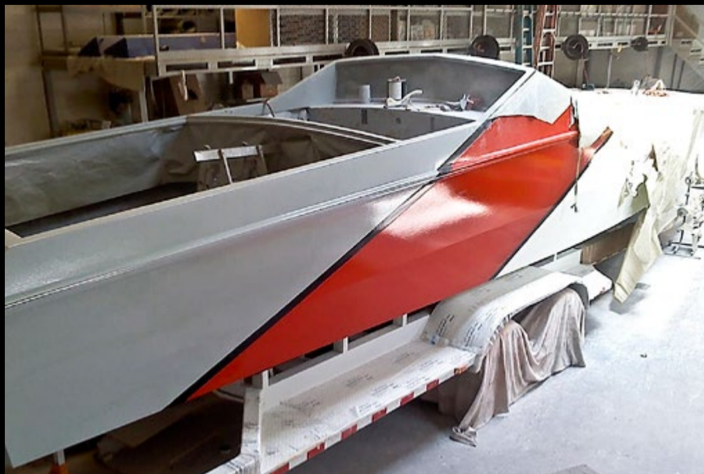
Hundreds of man-hours went into sanding and buffing the 41-foot Apache before it was turned over to Krazy Kolors to lay down the stellar candy red and white paint job on the “new” Straight Arrow .
