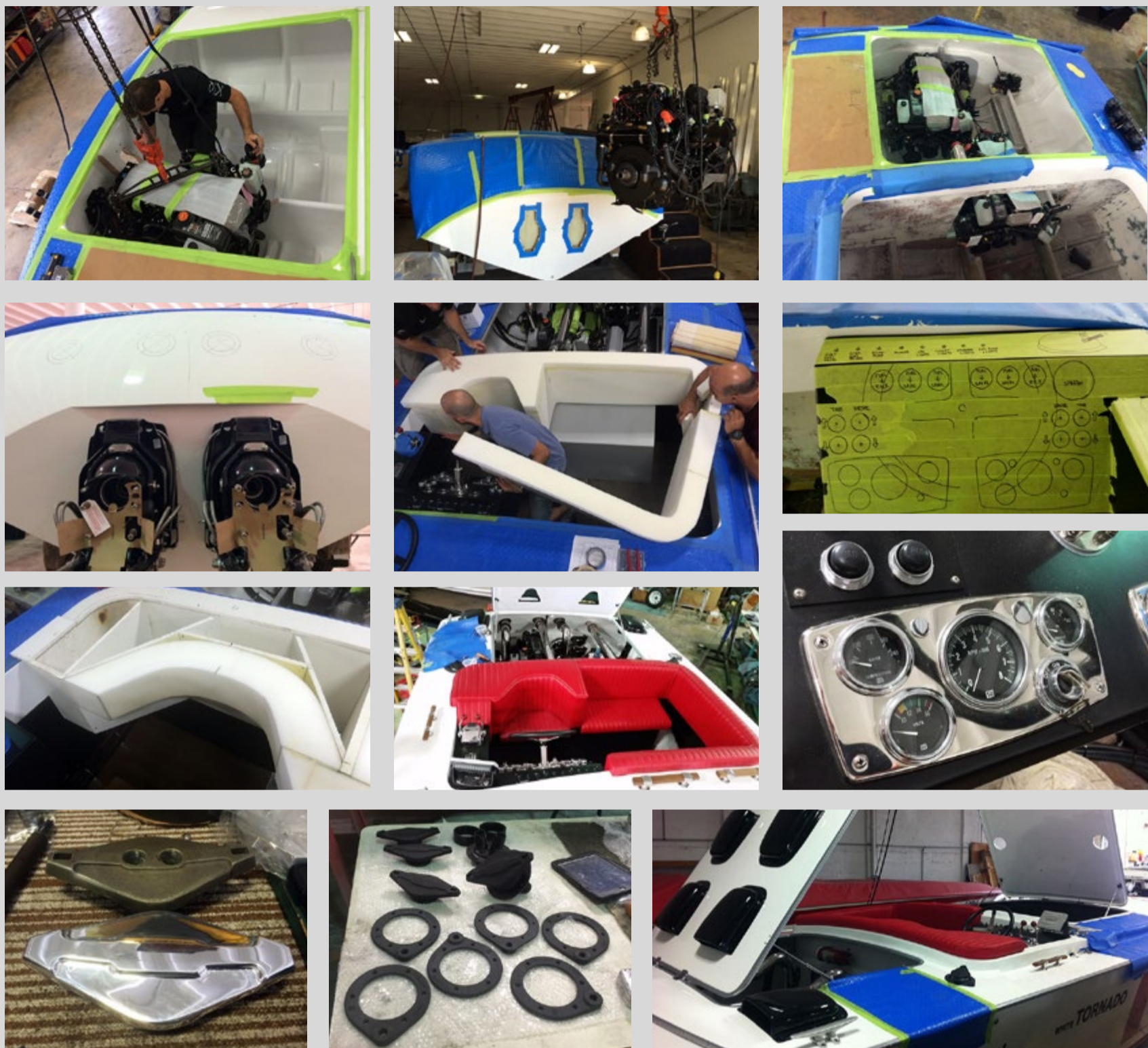
From rigging the twin Mercury Racing 520 engines and Bravo One XR drives to machining custom hardware, getting the helm station just right and working with Miami Prestige Interiors to execute the classic race-style cockpit, TNT Custom Marine put hundreds of hours into the restoration of the 50-year-old, 31-foot Bertram.
