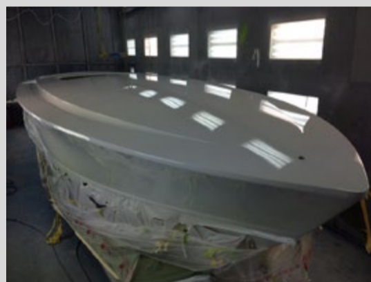
As shown in the top images, the 31-foot Bertram was a complete mess when Cadillac McDaniel purchased it. Fortunately the crew from Guardado Marine in Opa-locka, Fla., got its hands on the boat and gutted it, rebuilt practically everything, refinished it, painted it and sent it over to TNT Custom Marine to finish the restoration.
